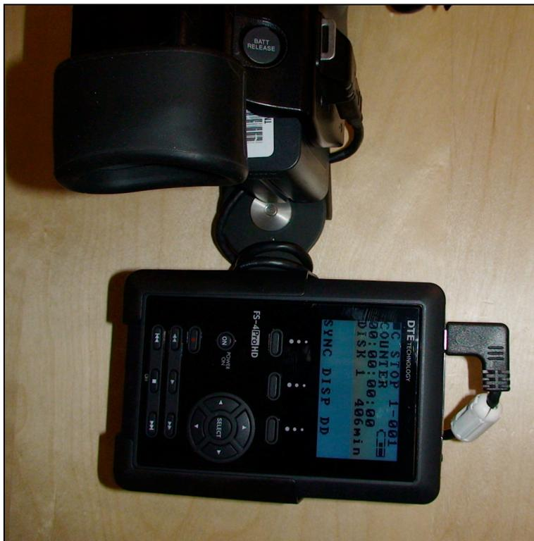
Notice the angle of the Firewire cable connector that is plugged into the FS-4ProHD. It is possible to connect this backwards, which will not record video to the Firestore drive. Make sure this Firewire connector is correctly installed (the connector has one rounded side and one flat side, so does the cable, they should match!).
