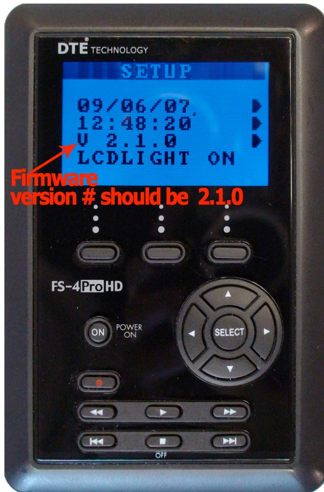
**FS-4ProHD Firmware version 2.1.0** provides video and audio sync and defaults to HDV recorded as a QuickTime (instead of m2t). Version 2.0.0 records the Audio being out of sync by 2 frames ahead of the Video and the HDV video defaults to M2T (not QuickTime).
