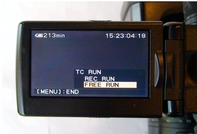
To allow recording the "Time Of Day" from the Sony Z1U to the Firestore drive, it is necessary to make two changes. 1) to set "TC RUN" to "FREE RUN"...
