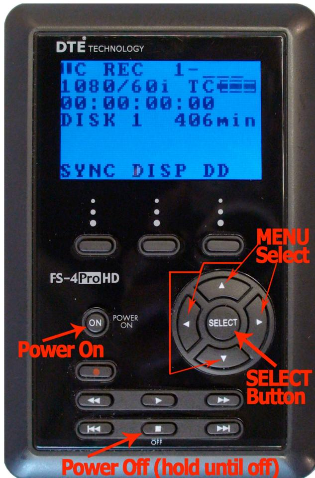
To power up the FS-4ProHD, hold the "POWER ON" button down for around one second and release. The Firestore drive should start up (the "release" of the button starts it up). To power off the FS-4ProHD, hold the "OFF" button down until you hear six "beeps" and until the Firestore powers itself off.
