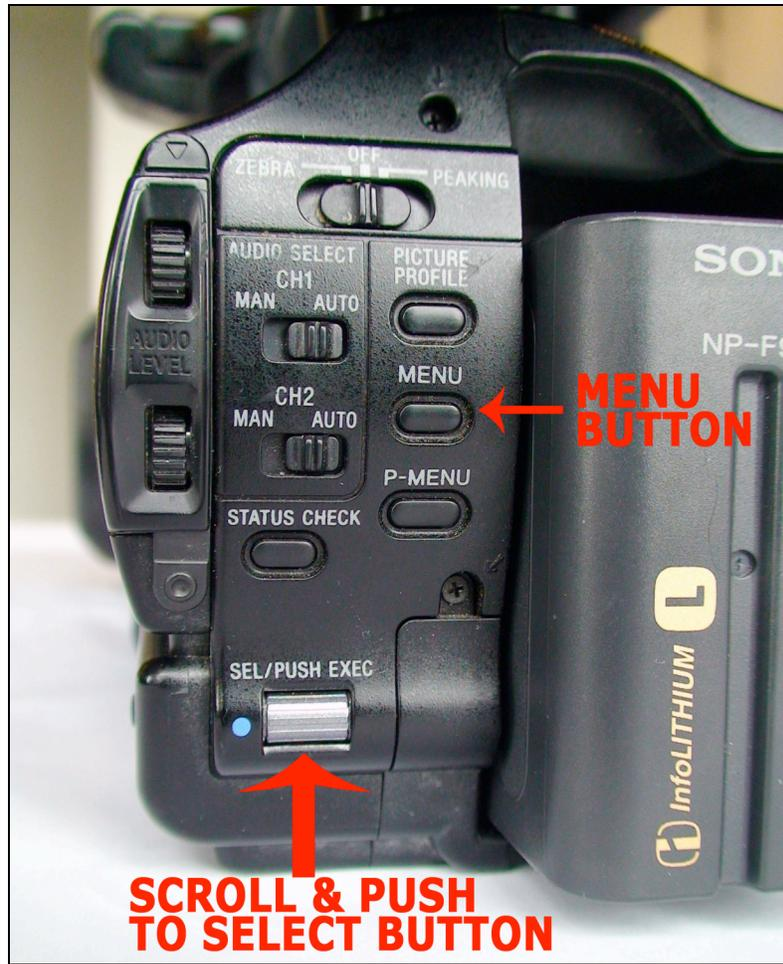
Using the Sony Z1U "MENU" button enters the Menu on the Z1U video display, using the roller/button on the bottom of the Z1U is how you scroll through menus and pushing in on that roller selects menu items.
