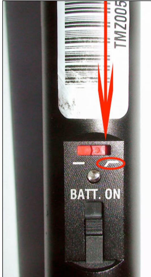
SENNHEISER SHOTGUN MICROPHONE - Push the RED switch to the right for roll-off (see image above).
