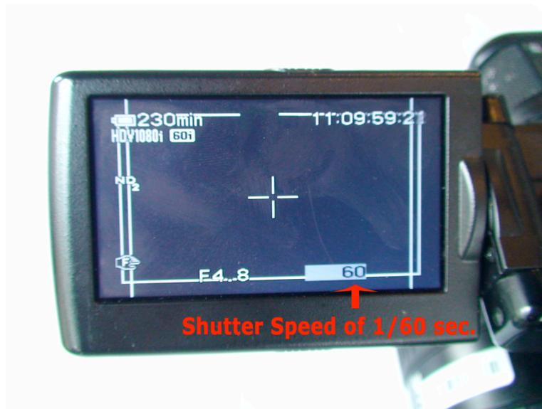
The Sony Z1U should have its shutter speed set to 60 (1/60sec.). 60 is the TMZ standard shutter speed. Do this by sliding the "AUTO LOCK / HOLD" slider to the center position, push on the "SHUTTER SPEED" button and using the roller wheel on the back of the Z1U, select the shutter speed of "60" (viewable in the Z1U display - above image). Push "AUTO LOCK / HOLD" slider to "HOLD" to lock the shutter speed.
