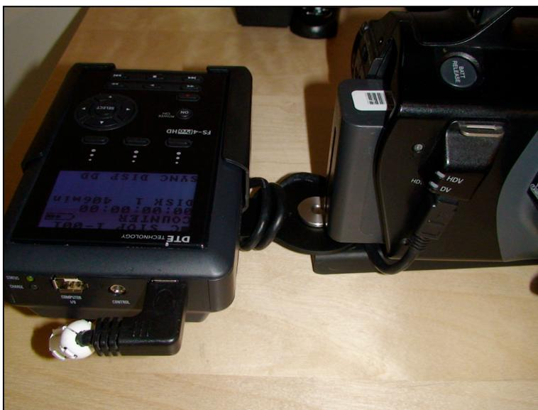
**It is very important** to wrap the Firewire cable around the mount (see photo) and push the cable under the battery and up into the Z1U camera (4 pin) Firewire input. This will "spring load" and force the cable into the camera to reduce the chance of the Firewire cable falling out, or being pulled out of the camera. The Firestore (6
