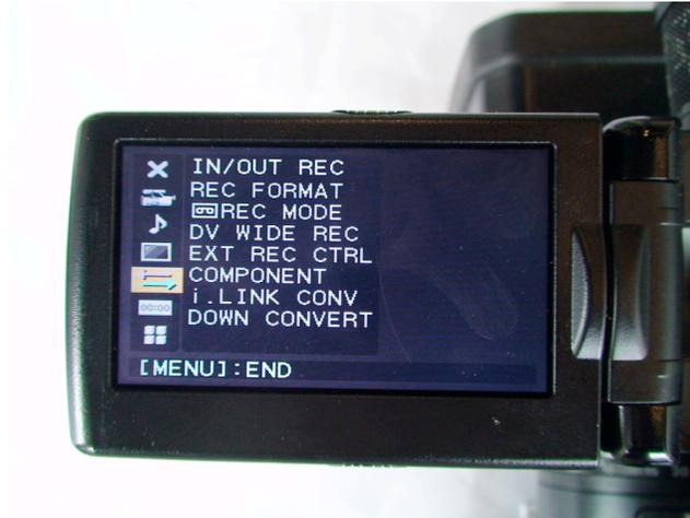
Using the roller wheel on the back of the Z1U, select "IN/OUT REC" menu ...
