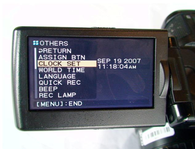
Set the "CLOCK SET" to the correct time and date, though this is not used for the "FREE RUN" time code, it is encoded into the Firewire data stream and can be recalled later for the correct time and date any HDV, or DV video is recorded.
