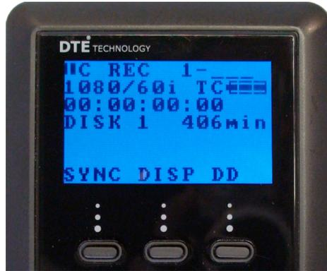
This is the first screen you see when you first power on the FS-4ProHD. There are three important buttons (shown in image) you will use in daily operation. They are the "SYNC", "DISP" and "DD" buttons (the physical buttons are on the case, just below the words in the display).
